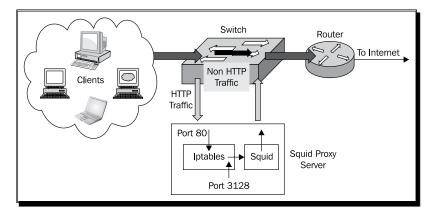
In the previous diagram, we can see that the switch is passing HTTP traffic to the Squid proxy server based on rules configured in the switch. All the non-HTTP traffic is directly forwarded to the internet.
