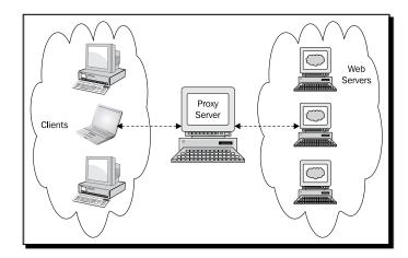
As seen in the preceding image, clients can't make direct requests to the web servers. To facilitate communication between clients and web servers, we have connected them using a proxy server which is acting as a medium of communication for clients and web servers.
