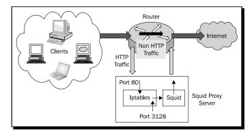
In the previous diagram, we can see that the router is passing all the HTTP requests to the Squid proxy server and all the non-HTTP traffic is going to the internet directly. A router can only modify the IP address of a packet. So, we must configure an IP packet filtering tool (iptables, ipfw) to redirect traffic on port 80 to the port on which Squid is listening.
