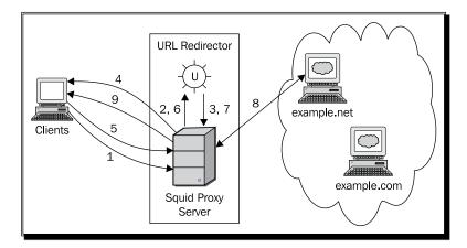
The previous diagram shows the flow of requests and responses using numbered steps. Let's try to learn what is happening at each step in the previous diagram:
