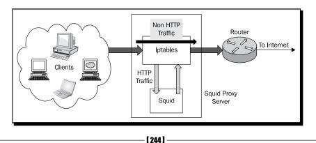
In the preceding diagram, we can see that we are not using any switch or router to direct HTTP traffic to the Squid server. Instead, all the traffic is passing through the Squid server and the iptables direct HTTP traffic to the Squid process, and passes the rest to the router connected to internet. This is the easiest of the three ways to achieve interception caching as we don't have to configure our router or switch, which is generally a relatively complex task.
