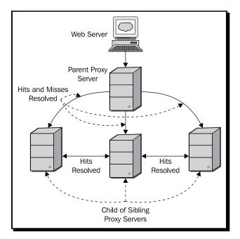
Siblings are the proxy servers at the same level in the tree structure. In a cache hierarchy, proxy servers use protocols like ICP, HTCP, Cache Digests, and CARP to identify a useful source. The other peering types are origin server, which is generally a special type of parent and multicast, which in essence is a special type of sibling.
